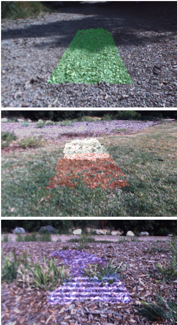
Fig. 5. Back-projected proprioceptive classifications. Top: Classification is invariant to lighting. Middle: Transition from grass (red overlay) to unknown-terrain class. Bottom: Region labeled mulch (blue overlay) but partly with low confidence (striped area) due to intervening grass. Another back-projected classification is in the left panel of Fig. 1.
